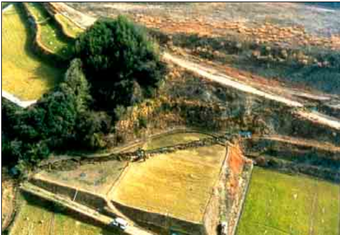
Figure A3.8 – Aerial view of the fault rupture on northern Awaji Island due to 17 January 1995 Kobe earthquake ( M_w 6.9). Photo courtesy of Y. Kinugasa.
