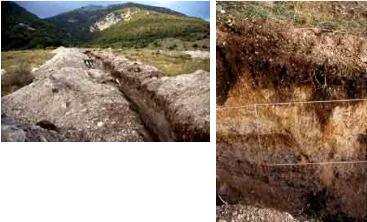
Figure A3.18 – Trench across a fault scarp along the Pollino active fault zone (located near the border between Basilicata and Calabria, Southern Apennines). No historical events are known in the area, but the trenches have revealed a Middle Age earthquake, with significant impact for seismic hazard (Michetti et alii, 1997). Photo E. Vittori.
