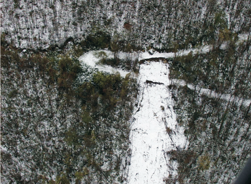
Figure 14: Translational slide evolving as a flow triggered on a bend of a forestry road, Cervinara Municipality (Campania Region), December 15, 1999
