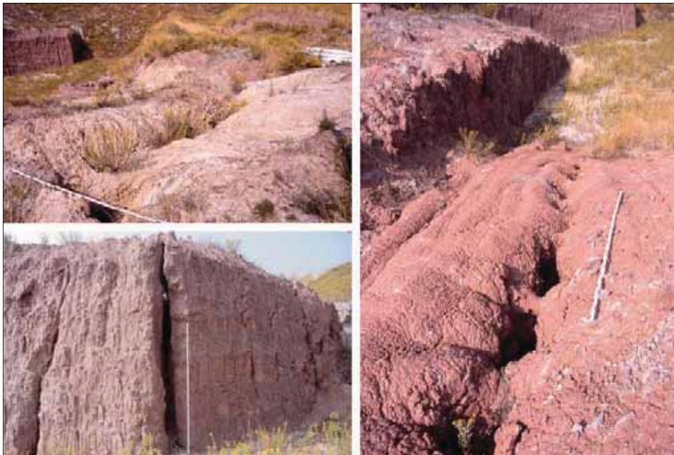
Fig. 4 - Common suffosion ( piping ) sinkholes developed upon fractures in mountain rextatic areas between Bologna and Modena Appennine.
