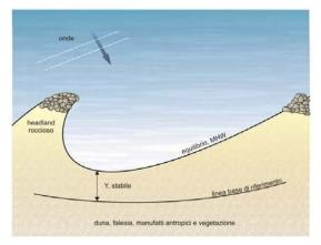
Figure 1.4.6 - Effects of a headlands built by natural blocks (APAT, 2007).
