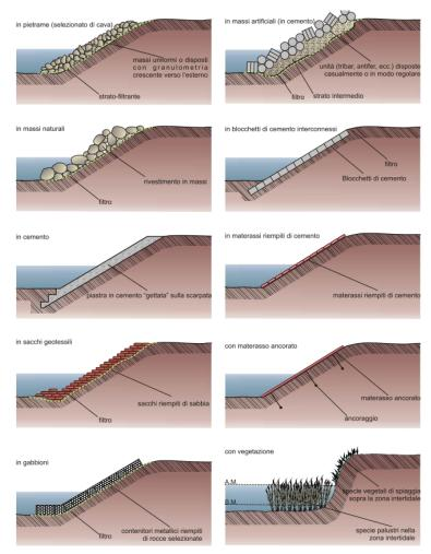
Figure 1.1.2 - Revetment types (APAT, 2007).
