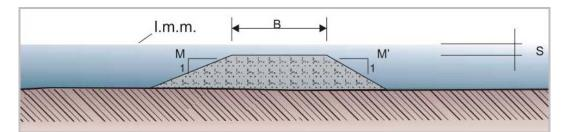
*Figure 1.3.2* - Scheme of a typical submerged breakwater (B= crest amplitude, S= submergence; M= seaward side slope; M' = landward side slope) (APAT, 2007).
