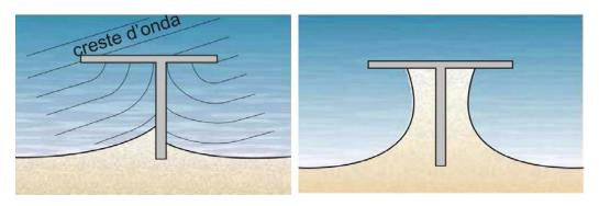
Figure 1.4.5 - Effects associated with T-shaped groynes (APAT, 2007).
