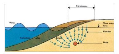
Figure 1.7.1 – Section of a drainage system (http://www.shoregro.com).
