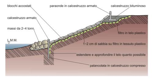
**Figure 1.1.1** – Scheme of an alongshore structure for low coasts with mild wave action. The armour is made of concrete slabs mutually interlocked and resting on a base provided with a filter, of a protection at the base and of a breakwater at the top (APAT, 2007).
