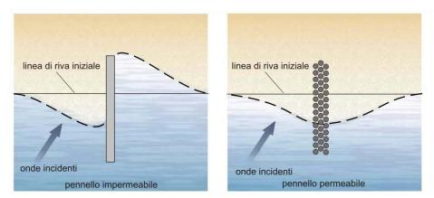
Figure 1.4.2 - Effects of impermeable (left) and permeable (right) groynes (APAT, 2007).
