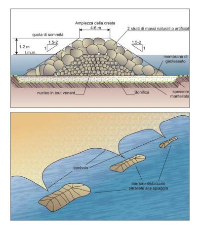
*Figure 1.3.1* - *Emerged detached breakwaters scheme (above); effects induced by emerged breakwaters (below) (APAT, 2007).*
