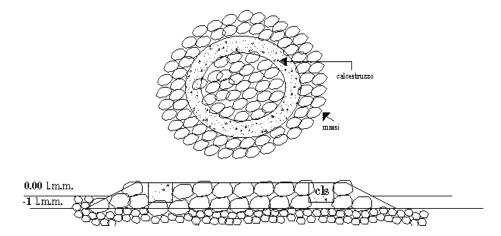
Figure 1.3.3 - Scheme of an island-platform: plain-view (above); sectional view (below) (Tuscany Region, 2007).
