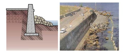
Figure 1.1.4 - Vertical concrete seawall with a natural rock protection at the toe (APAT, 2007).
