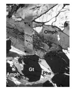
Figure 56 - Photomicrograph of a preserved portion of palaeocrysts in eclogite E22h seen under crossed polarisers. The superposed inlet is a concentration map showing rising Fe contents by increasingly lighter grey tones. Image width is 2.7 mm.
