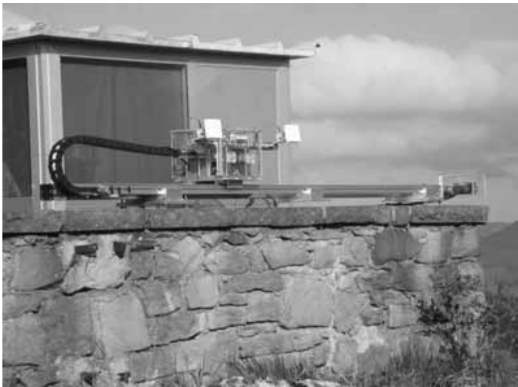
Figure 10 - LISA is a ground-based portable apparatus consisting of a motorised sled, carrying a transmitting and a receiving antenna, which slides along a straight rail, about 3 m long. The synthetic aperture is realised by acquiring raw data at selected positions along the rail.. Photo by Nicola Casagli, 2003.
