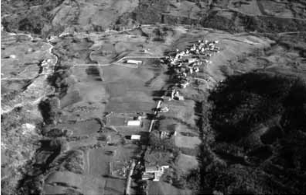
Figure 3 - The flatter, wider and apparently stable parts of the Apennine slopes where many villages grew up over the last few centuries often are the exposed feet of very large, dormant landslides. Photo by Giovanni Bertolini, September 2002.
