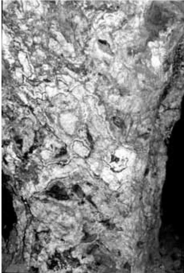
Figure 4 - Geodic dolomite with generation I (dark grey) and generation II (white, filling tension gashes and dilatational cracks). San Giovanni mine, lev. -60 (hammer = cm 35) (from Boni et al., 2000)
