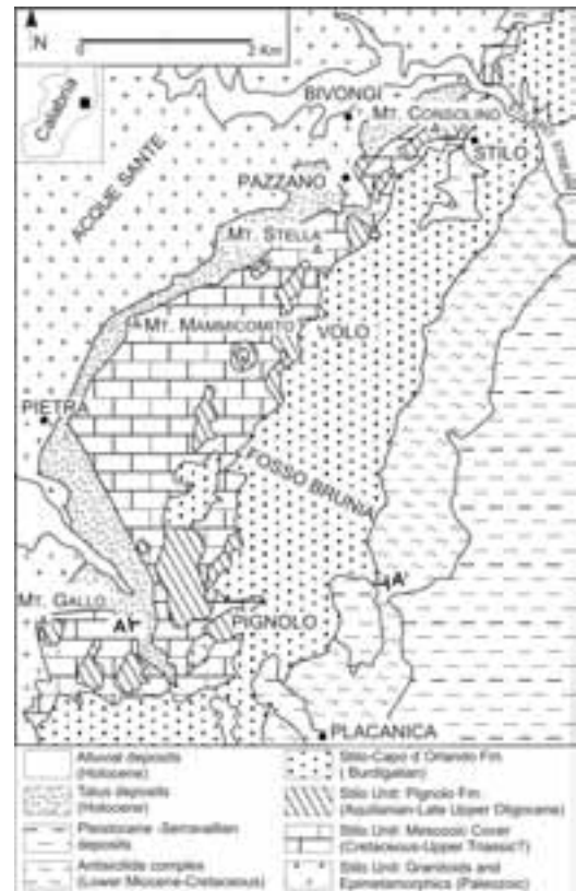
Figure 29 - Geological map of the Monte Consolino-Monte Stella-Monte Gallo ridge (modified after Bonardi et al., 2003). A-A' = location of the section of fig.33.
