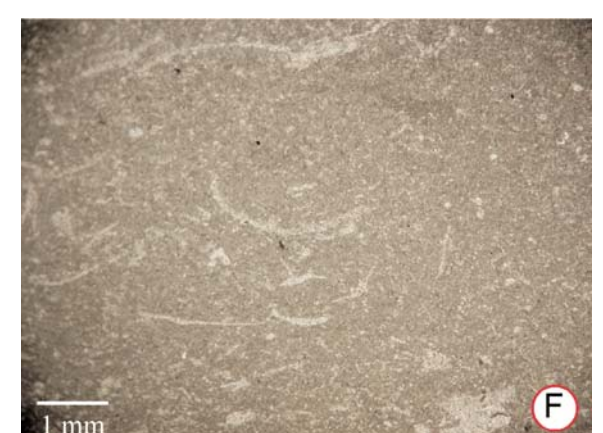
Thin-section microphotograph, in transmitted light, of Calcare nodulari a Saccocoma ed Aptici (NAS). This wackstone with Saccocoma remains (pelagic crinoid) come from one isolated outcrop, to the north of S. Angelo Romano, which directly overlies the Calcare massiccio Fm.
