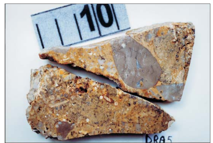
Fig. 8 - Floatstone composed of lithoclasts and bioclasts, dredged from the substrate in the Bocca Piccola area. Clasts of very different shape, size and composition are embedded in a reddish calcareous matrix. Scattered black dots correspond to iron-manganese concentrations. Diffuse perforations are due to biologic activity (bioerosion).
