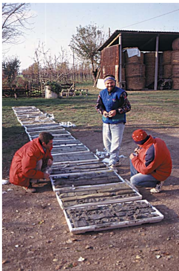
Fig. 12 - The surveying crew of the subsurface geological map conduct high-resolution sedimentary and stratigraphic analyses on core sediments retrieved from borehole 240-S2 (to a depth of 170 m), in order to reconstruct the stratigraphic and paleoenvironmental evolution of the Forlì plain over the last 400-500 thousands of years.
