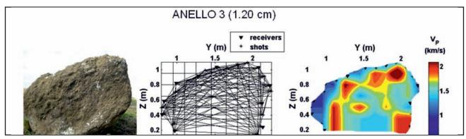
Fig. 19 – Seismic tomography on a Moai of the Easter Island. Different color indicates seismic wave velocity (Vp) showing area of low velocity and then less resistant (Courtesy Prof. L: Orlando, University of Rome – Italy).
