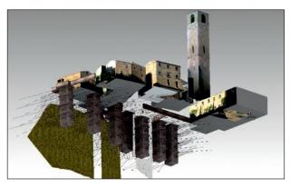
Fig. 23 – The innovative consolidation work for the stabilization of rock slope in Civita di Bagnoregio: Anchors and bolt realized from structural wells.
