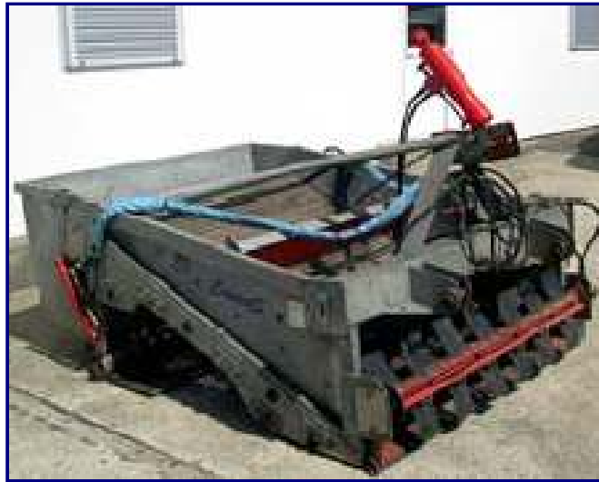
Figure 5. A specific device normally used to clean touristic sandy beaches (source www.cedre.fr )
