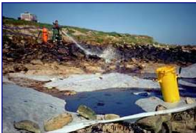
Figure 1. A low pressure water pump utilized to collect bulk oil (source www.cedre.fr )
