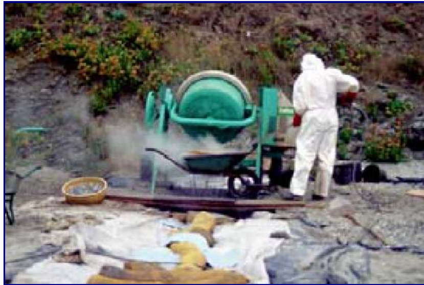
Figure 7. A mortar mixing machine utilized for cleaning pebbles contaminated by hydrocarbons (source CEDRE, www.le-cedre.fr )
