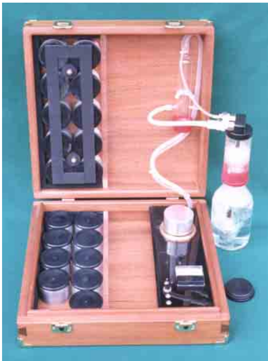
Figure 4 : Photograph of the degassing portable system.
