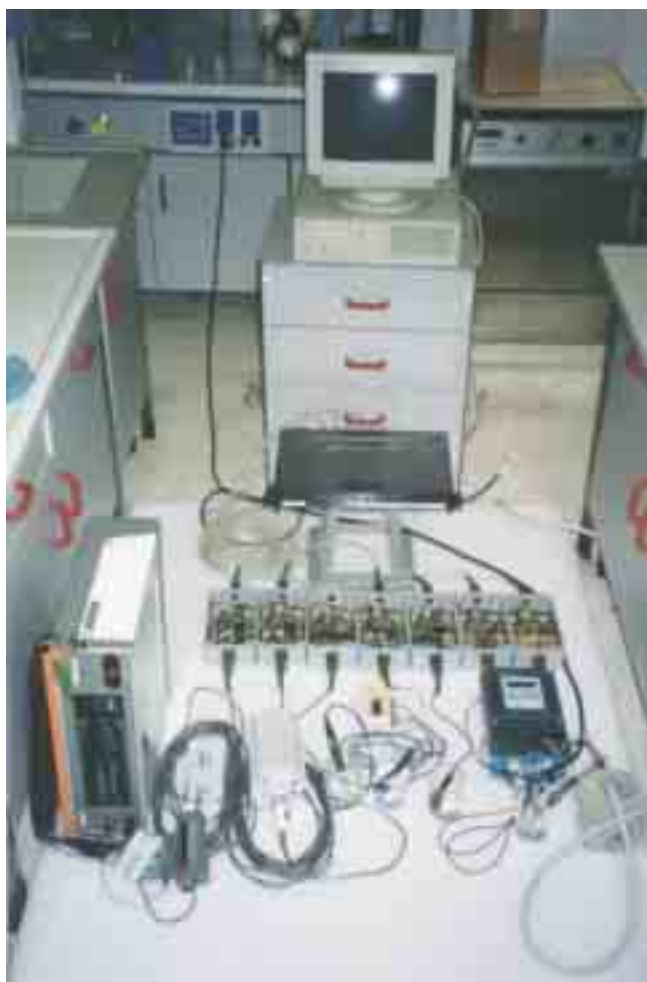
Figure 1: The Geochemical Monitoring System II prototype (GMS II) designed and assembled by ING. Consisting of a PC-IBM compatible computer (2 serial port equipped, Window95 available), an ING-designed serial collector-multiplexer . (black box, in front of computer) serial port collector, A/D signal conditioning systems (eight up to date) for the available sensors. The sensors shown are from left: He-mass spectrometer ( Alcatel™ ASM 100 HDS continuous He flux detector), atmospheric pressure, air temperature, electrical conductivity in groundwater ( B&C Electronics™ ), CO 2 partial pressure in groundwater ( Idronaut™ ), pH, Eh and temperature ( Endress & Hauser™ ). The Radon in groundwater signal has a serial port available, within the serial collector-multiplexer .
