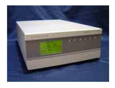
Monitor Europe ML 9830 Carbon monoxide (CO) Analyser is a Non-Dispersive Infrared (NDIR) photometer, which uses Gas Filter Correlation (GFC) to measure low concentrations of CO accurately and reliably.
