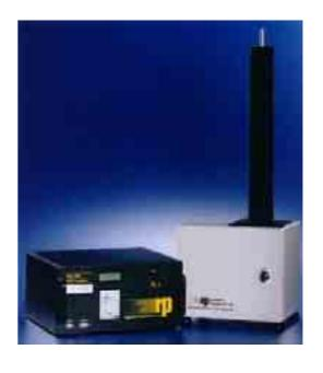
The Series 1400a monitor incorporates an **inertial balance** that directly measures the mass collected on an exchangeable filter cartridge by monitoring the corresponding frequency changes of a tapered element.
