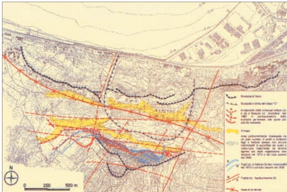
Figure 2. Main geomorphic features in the area of the Ancona landslide, including the location of fractures and flexural scarps most likely generated during the 1972 earthquake sequence (modified after Cotecchia, 1997).
