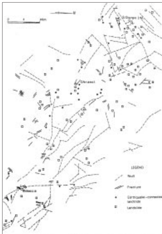
Fig. 3. Pattern of fractures and landslides induced by the 1980 Southern Italy earthquake between S. Giorgio la Molara and Bisaccia
