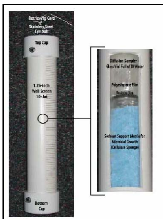
Figura 11.2- MICRO-Trac (Modular In Situ Community Response Outfit) da WRSC 2006.
