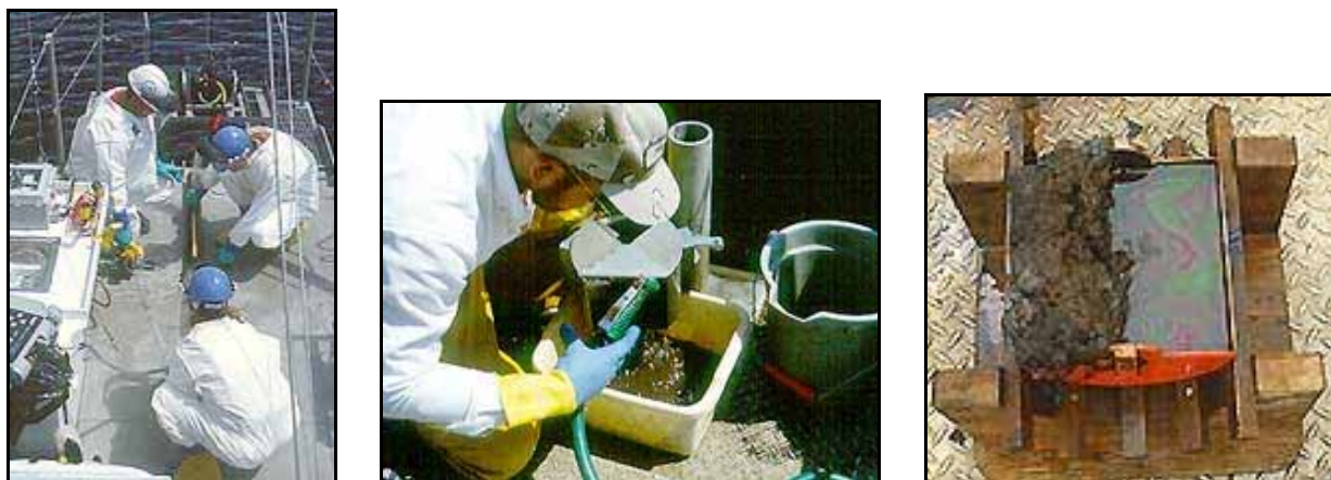
Figure 4. Collection of sediment samples from the St. Louis River AOC [left to right: collection of a sediment core from Slip C, collection of sediment for enumeration of benthic invertebrates, and collection of sediment for bioaccumulation testing (note the oil sheen)].
