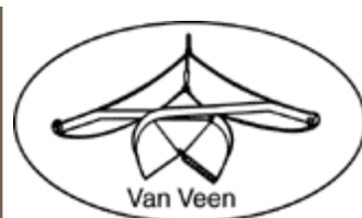
Figure 6. Van Veen grab sampler.
