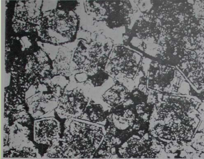
Fig. 7-10. Dolomitic limestone with complex texture. The dolomite rhombohedrons are composed of core and thin rim. The cores are composed of very fine-grained calcite with dolomite background, whereas the rims are pure dolomite. Areas between rhombohedrons are filled with medium-grained calcite. Insoluble residue: 1.70%, \text{CaCO}_3 : 75.37%, \text{CaMg}(\text{CO}_3)_2 : 22.88%. Upper Carboniferous, Samarskaya Luka. (After Khvorova, 1958, fig. 175, p. 127.) Diagenetic dolomite, later altered during epigenesis; \times 45 .
