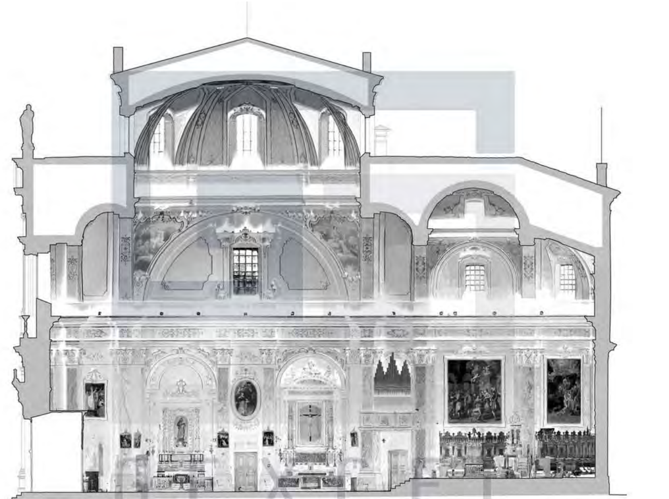
Internal cross section with reflectance information (Software: JRC 3D Reconstructor) | Sezione interna con riflettanza (Software: JRC 3D Reconstructor)
