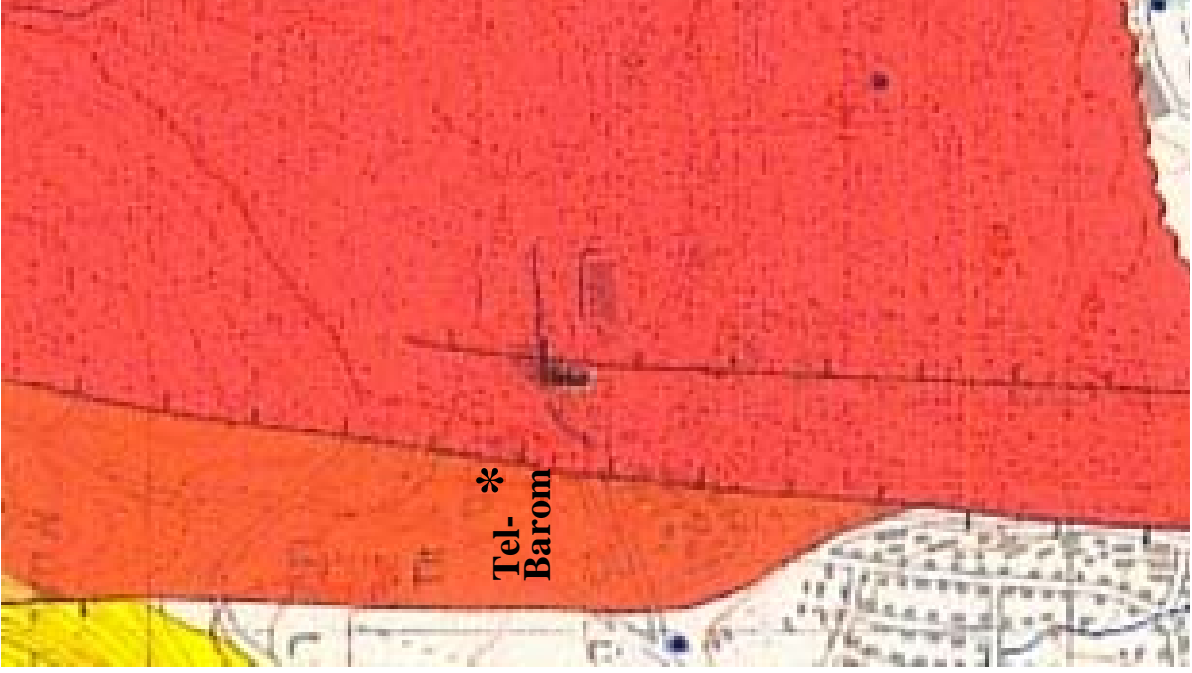
Figure 19: An excerpt from the geological Map of Metulla, Sneh and Weinberger, 2004. Orange - Paleocene Taqiya Formation. Yellow - Neogene Kfar Giladi Conglomerate. Red - Pleistocene Hasbani Basalt The light triangle marks the FZW active seismic experiment.
