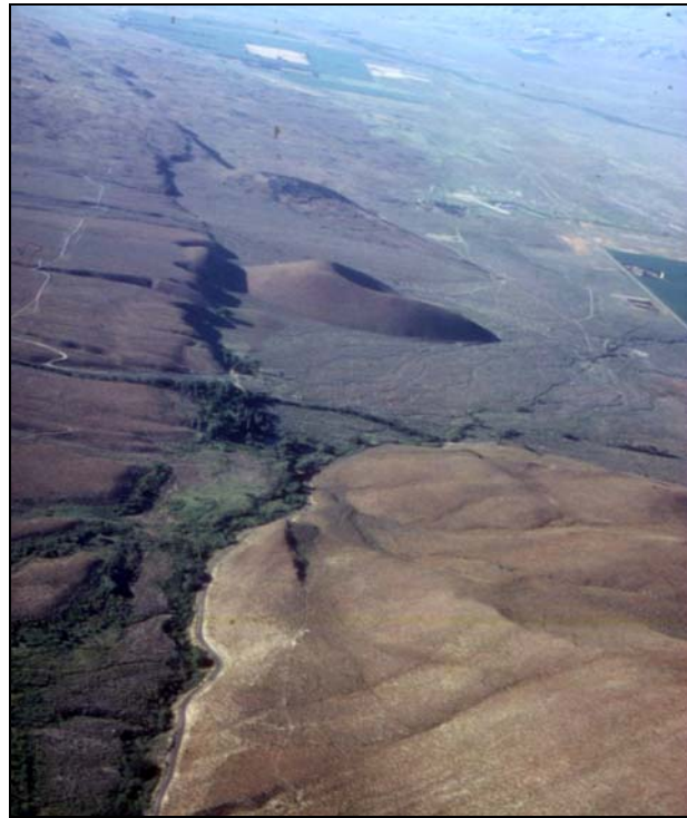
Figure a – Oblique aerial view of the Owens valley fault zone (eastern California), affected by more than 110 km of surface faulting during the March 3, 1872 earthquake ( M_s 7.6) (Vittori et al., 2003). Photo E. Vittori.
