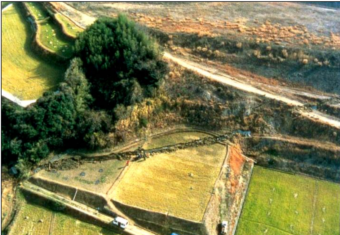
Figure h – Aerial view of the fault rupture on northern Awaji Island due to January 17, 1995 Kobe earthquake ( M_w 6.9). Photo courtesy of Y. Kinugasa.
