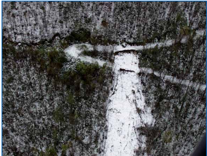
Figure 7.18: Anthropic contributing factors - Translational earth slide flowing near a hairpin bend in a forest road, Cervinara (AV) 15/12/1999 19
