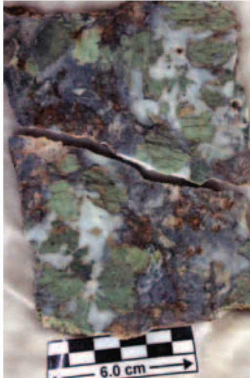
Figure 35 - Crepin: completely eclogitized gabbro. Pyroxene is green, plagioclase white, olivine (transformed to talc) is brownish. Note coronitic rims developed between the different microdomains.
