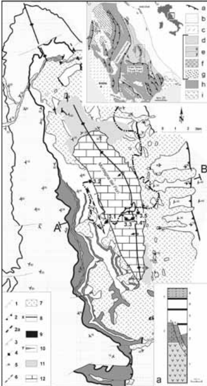
Figure 3.1 - Structural sketch map of the Montagna dei Fiori. The inset shows the tectonic sketch of the outer zones of the Central Apennines. The key to symbols is in Figure 1.1.: 1) Normal fault; 2) Thrust; 2a) Laga Detachment; 3) Backthrust; 4) Anticline axial trace; 5) bedding; 6) Itinerary and location of the stops (3.1 – 3.5); 7) Quaternary continental deposits; 8) Messinian Laga Fm.; X) Gypsum-arenitic layer; 9) Tortonian-Messinian Marne a Pteropodi Fm.; 10) Burdigalian-Tortonian Marne con cerroghna Fm.; Y) Calcareoclastic deposits; 11) Eocene-Oligocene Scaglia Cinerea Fm.; 12) Lower Lias-Eocene neritic-pelagic succession. A-B Trace of cross-section in Figure 3.2. a) Stratigraphic section of the Umbria-Marche succession. 1) Anidriti di Burano (Upper Trias); 2) Calcari e marne a Raethavicula e Calcare Massiccio (Upper Trias-Lower Lias); 3) Corniola, Rosso Ammonitico and/or Calcari e marne del Sentino (Upper Sinemurian-Aalenian); 4) Formazione del Bugarone (Pleisbachian-Lower Tortonian; in the condensed succession); 5) Calcari e marne a Posidonia, Calcari diasprini umbro-marchigiani, Maiolica, Marne a Fucoidi (Bajocian-Lower Cenomanian); 6) Scaglia bianca, rossa e cinerea (Middle Cenomanian-Oligocene); 7) Bisciario, Scheliet, Marne con cerroghna, Marne a pterapodi (Aquitanian-Messinian p.p.); 8) Turbiditic siliciclastic deposits (Burdigalian p.p.-Messinian). The heavy lines represent: Rosso Ammonitico, Marne a Fucoidi and Scaglia cinerea-Marne con cerroghna Fms, from older to younger respectively.
