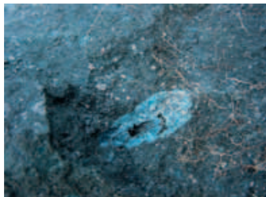
Figure 19 - Large phenocryst of häüyne (lazurite) in the Melfite (the crystal length is 4 cm).
