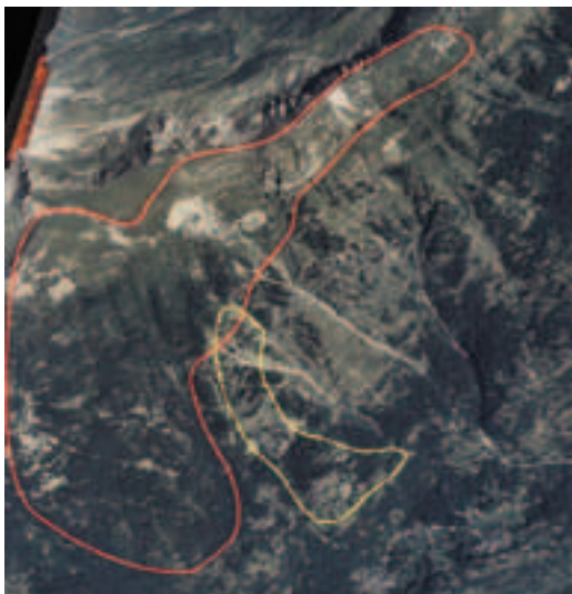
Figure 39 (left) - General overview of the Clot Brun large-slope instability: DSGD (red) and landslide (yellow).
