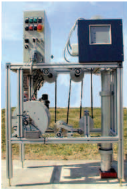
Figure 15 - Automatic Inclinometer System instrument.
