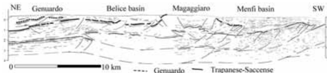
Figure 28 - Geoseismic interpretation of the section (a) in Figure 27, showing the structural setting of the Monte Magaggiaro antiformal stack thrusting over the Belice and Menfi basins.
