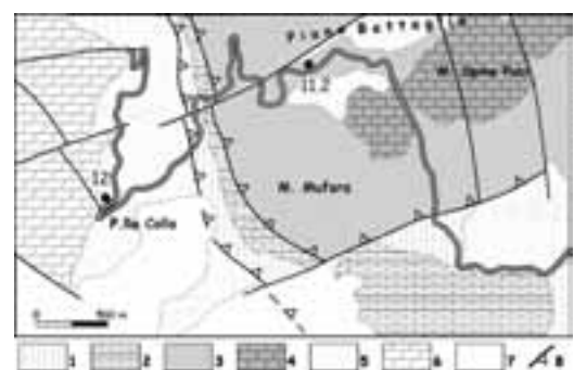
Figure 48 - Simplified geological map of the Portella Colla area. Marls and limestones (1), Mesozoic dolomites (2) (Quacella Unit). Triassic-Liassic (3) and Jurassic-Cretaceous platform carbonates (4) pertaining to the Panormide tectonic Unit. Numidian Flysch (5) and Imerese basinal carbonates (6) (Monte dei Cervi Unit). Debris (7). Mod. from Abate et alii (1982).
