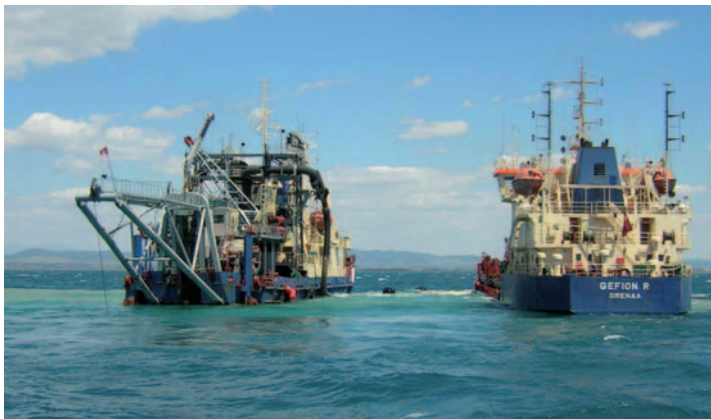
Figure 9.4: Some phases of relict sand dredging off Montalto di Castro (Lazio) 9
