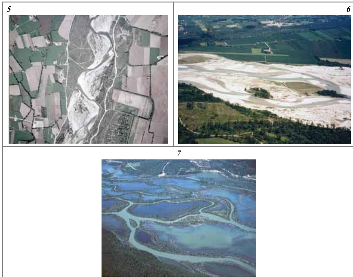
Figure 6 (continued) – Examples of morphologies of semiconfined and unconfined channels. (5) Wandering; (6) braided; (7) anastomosing (the islands and floodplain are inundated).
