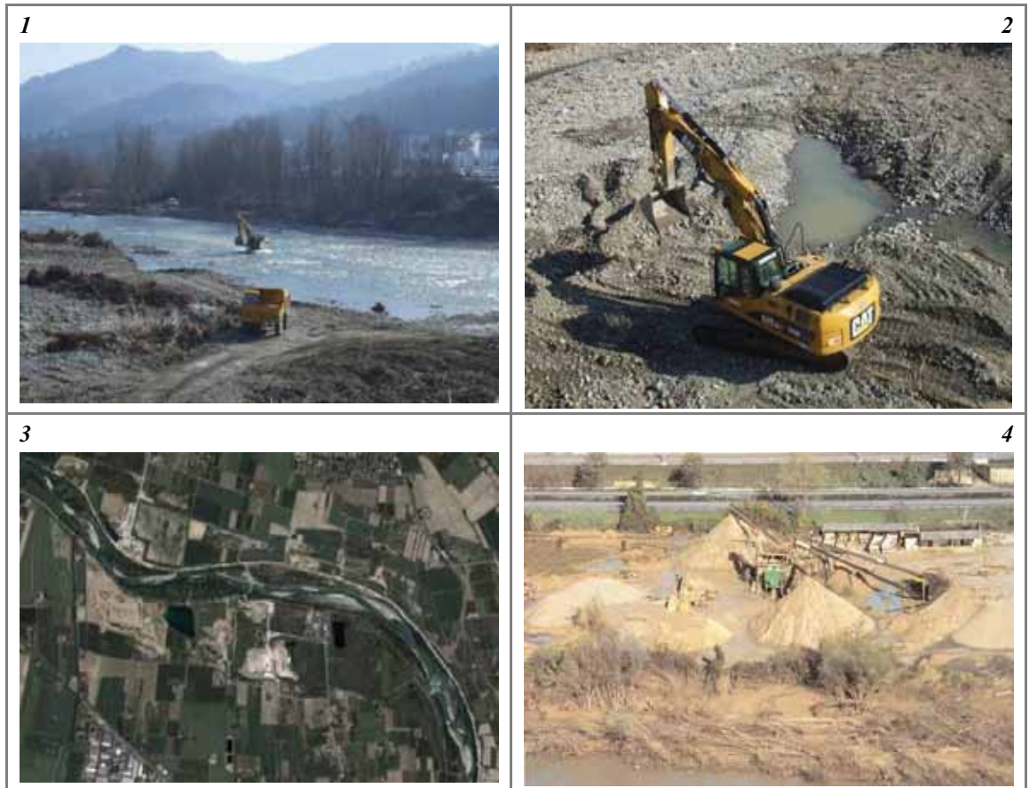
Figure 75 – Sediment removal. (1) and (2) Recent and present activity; (3) and (4) indirect indicators of intense past activity are the presence of mining sites. A signification to Class B or C depends on the extension of the activity ( localized or widespread), in the case of confined channels, and on the intensity of the mining activity either in the past and in recent times, in the case of semi- and unconfined channels.
