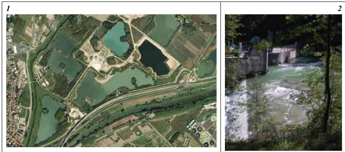
Figure 58 – Other structures (besides those defined for A1) that can cause an alteration of discharges within a reach. (1) Retention basins; (2) discharge abstraction.
