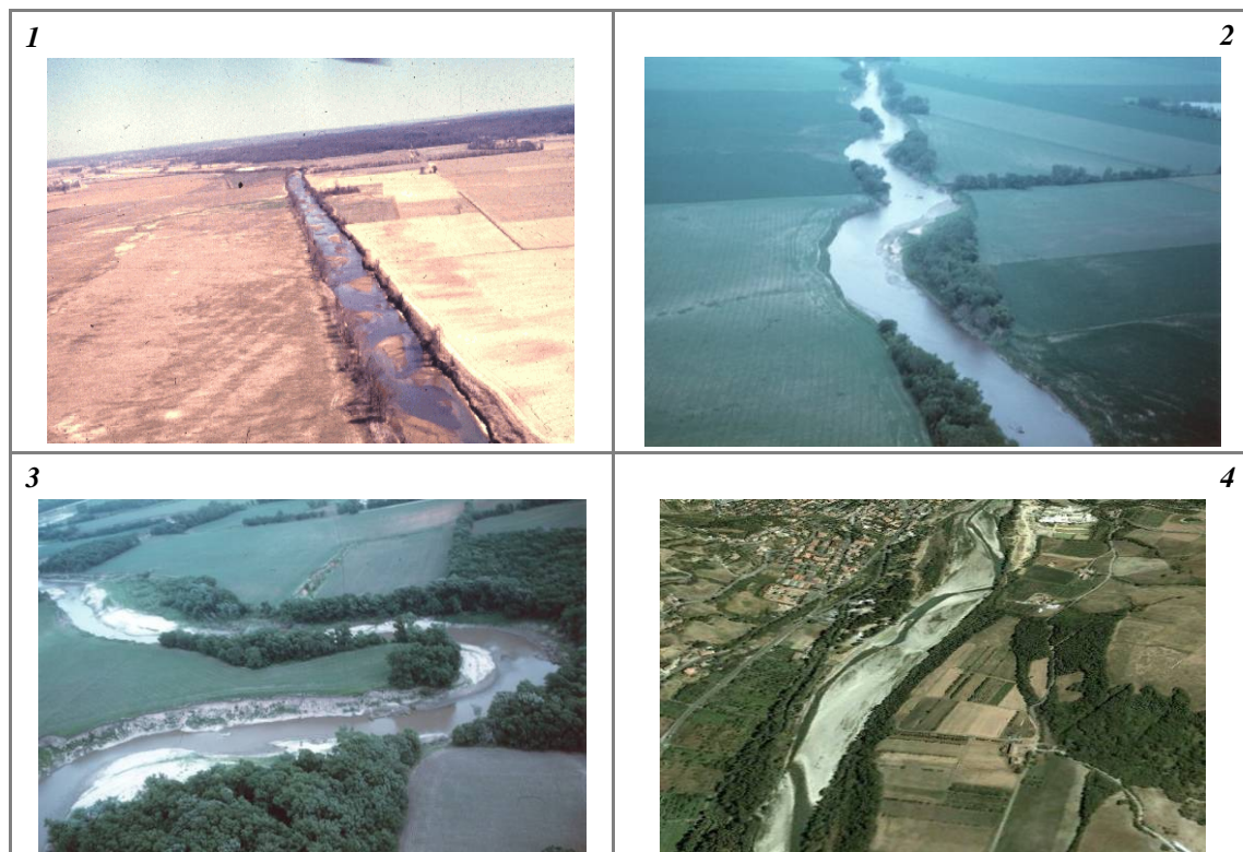
Figure 6 – Examples of morphologies of semiconfined and unconfined channels. (1) Straight; (2) sinuous; (3) meandering; (4) sinuous with alternate bars.
