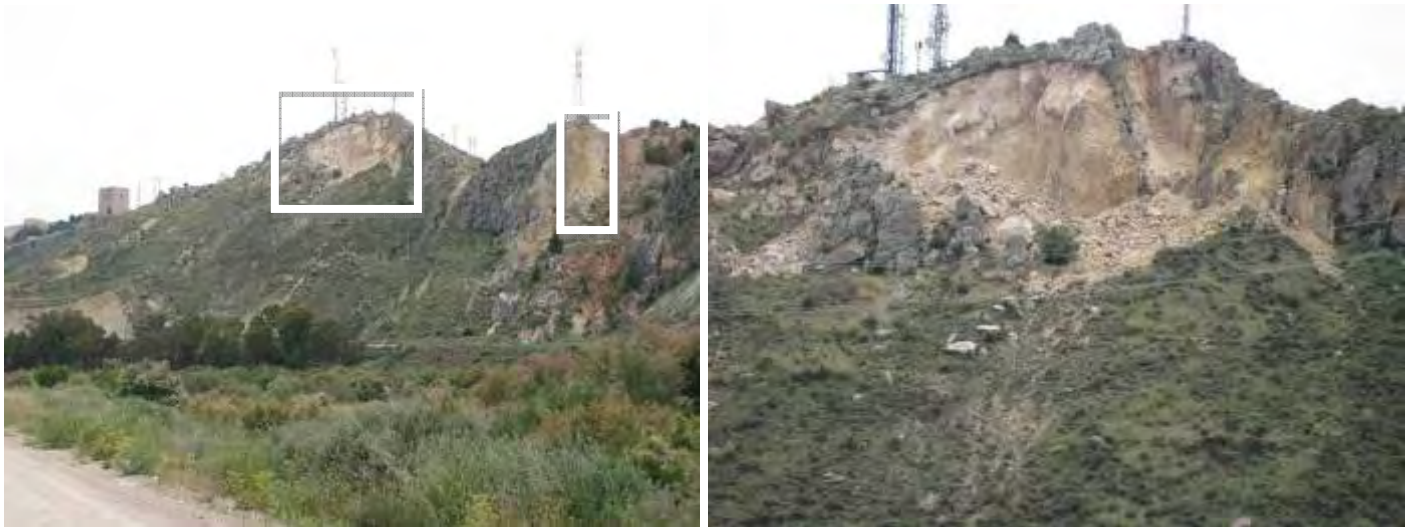
Figure 4.4.1a: Rock-falls and debris on the summit of the north slopes of the Pantano de Puentes road. Their attribution to the earthquake is presumed. The westernmost one (on the right on the first photo) corresponds in part with a previous instability.
