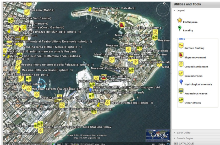
Fig. 2: EEEs induced by the December 28, 1908 Messina Straits, Italy, earthquake in the area of the Messina harbour. If information from contemporary sources is very precise, it is possible to use the EEE Catalogue also for local seismic microzonation.
