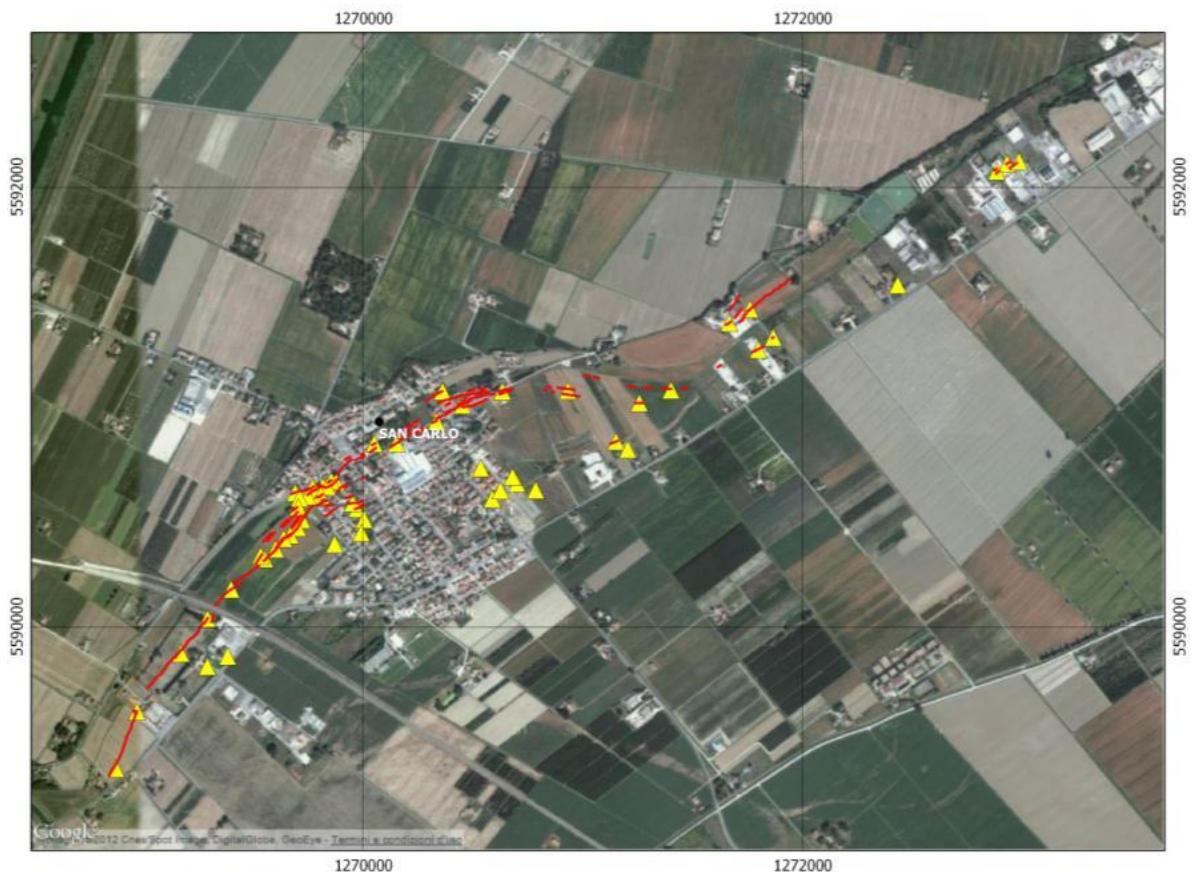
Fig. 3. San Carlo (Sant'Agostino): liquefactions and ground ruptures were distributed on a NE-SW trending elongated area located on an ancient embankment of the Reno River.
