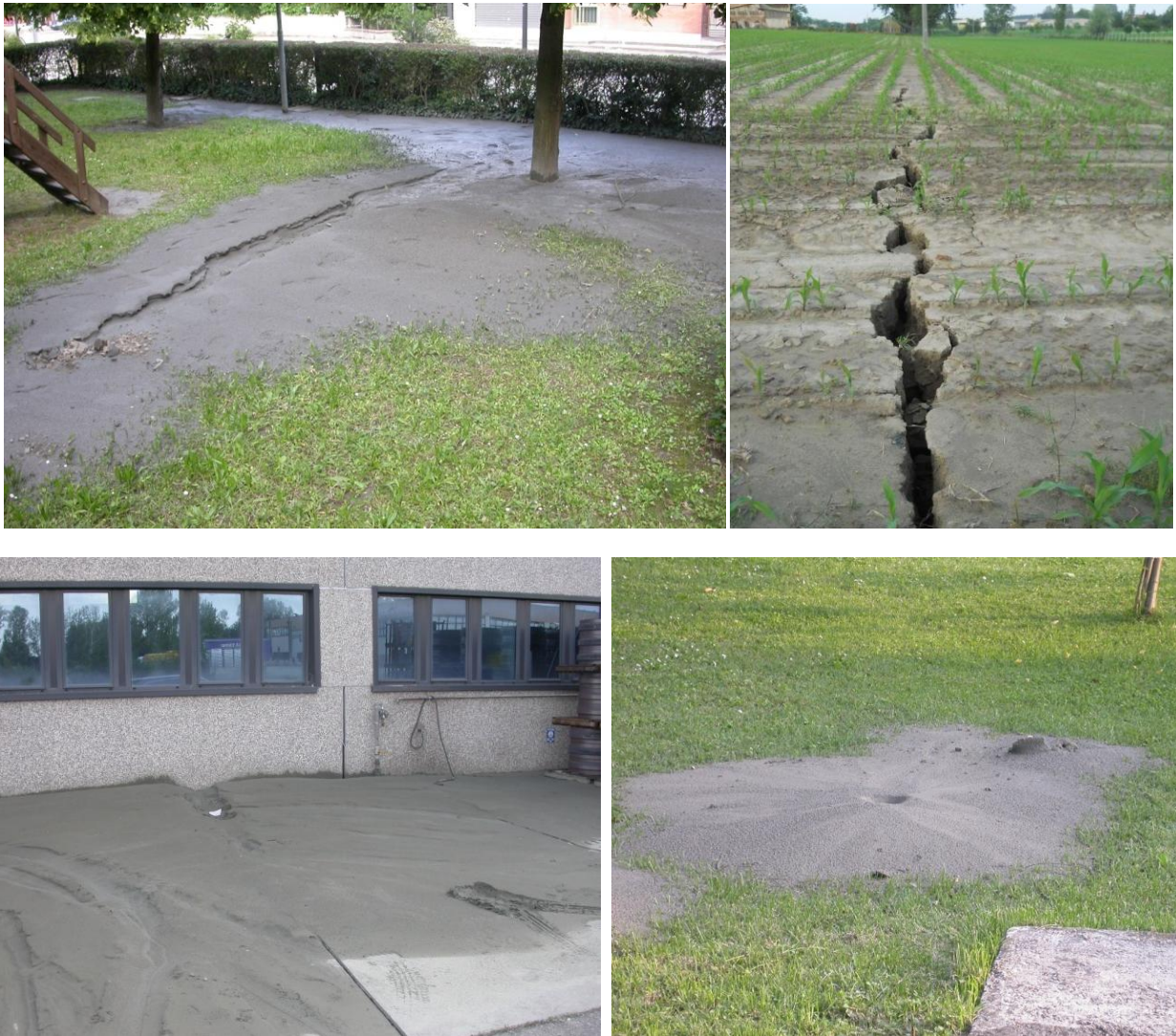
Fig. 6 – Mirabello: ground ruptures and liquefactions affected farmed lands, public and private gardens and industrial settlements.
