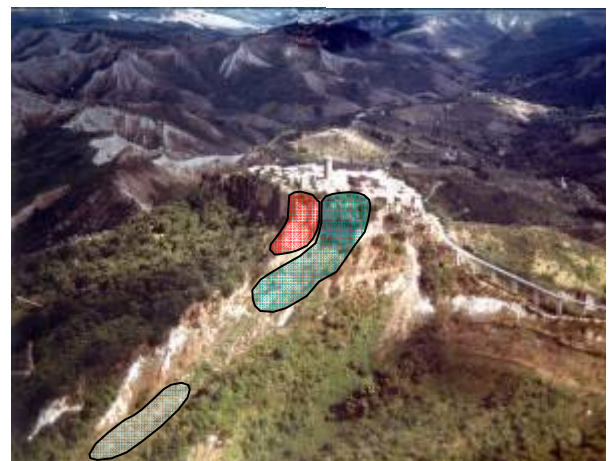
Figure 9. The three major areas of instabilities considered relevant for the future evolution of the cliff. From top-left “Casa Greco”, top-right “Cavon Grande”, bottom is the tuff debris.
