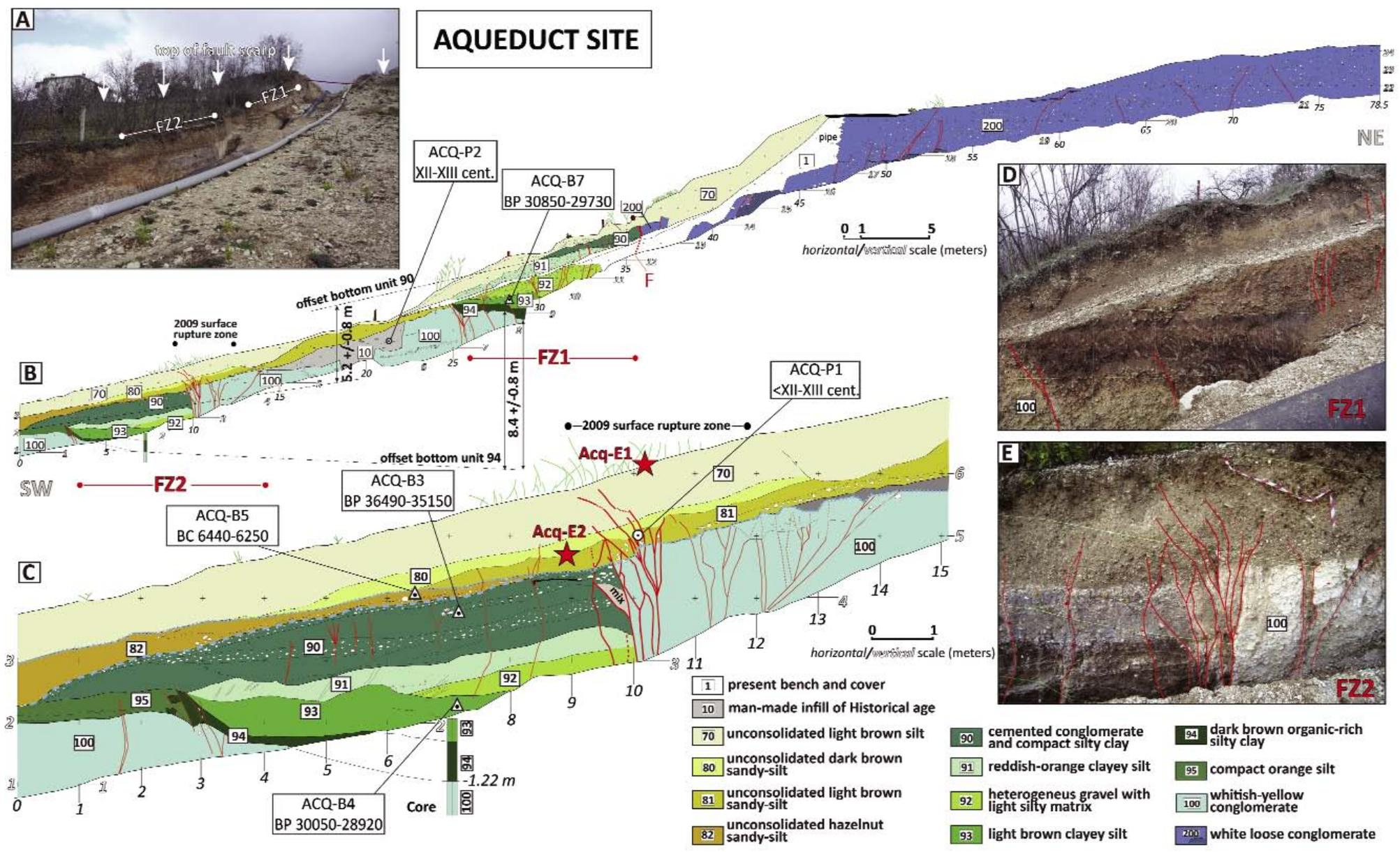
Fig. 51 - Aqueduct site trench (after Cinti et al., 2011). **a)** excavation along the Paganica sector crossing the 20 m-high cumulative scarp. **b)** and **c)** detailed log of the NW wall of the trench; **d)** and **e)** view of the main fault zones. At this site, the 2009 ruptures occurred at the base of the scarp on the fields and tarmac road adjacent to the pipeline. In coincidence of fault zone 2 (FZ2) the 2009 ruptures produced diffuse deformation accompanied both by cracking and warping.
