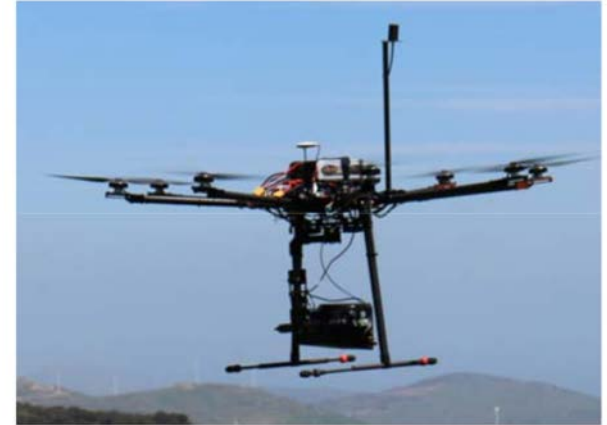
fig. 1 – Oben's octocopter carrying the LIDAR
