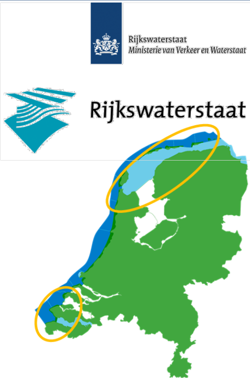
Figure 1. The boundaries of the coastal foundation and the coastal system in the Netherlands. Encircled are the areas with high sediment demand.
