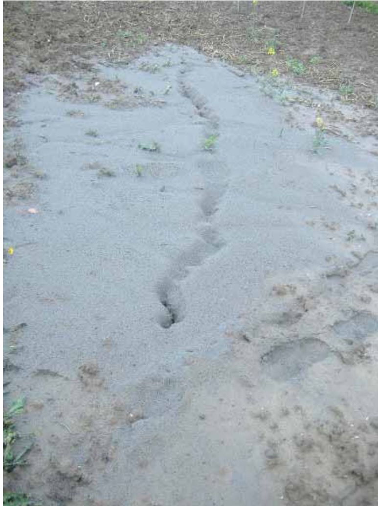
Fig. 41 – Mud/sand volcano near Vittorito (courtesy by G. Pipponzi, AdB Abruzzo),
