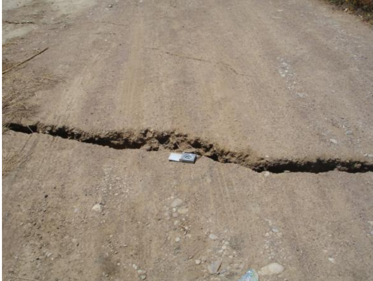
Figure 9. Surface rupture parallel to the coastline associated with liquefaction at Kato Achaia.
