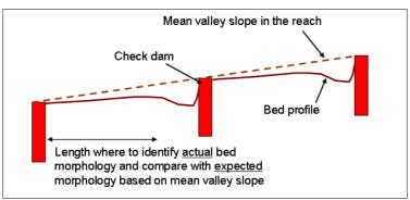
*Figure 34* – Bed configuration and valley slope. Rule for the measurement of the mean valley slope of the reach in the presence of structures (check dams) and to identify the length of analysis of bed morphology.
