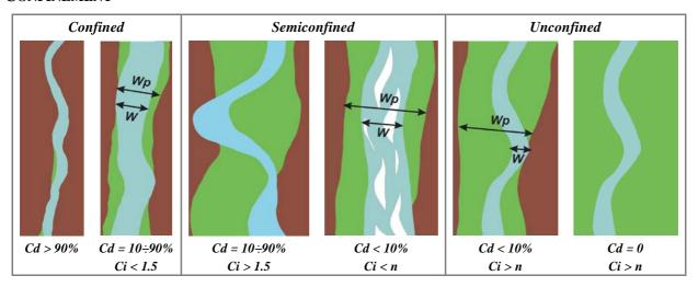
**Figure 3** – Confinement classes. In green: alluvial plain; in brown: hillslopes (or ancient terraces). Cd: confinement degree; Ci: confinement index = Wp/W, where Wp: alluvial plain width (including the channel) and W: channel width.
