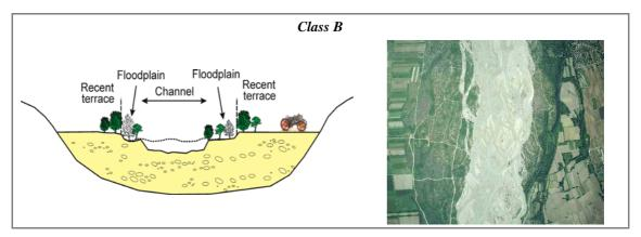
Figure 27 – CASE 3: the channel is moderately incised and slightly narrowed compared to 1954. Vegetation corridor is continuous and wide (F12 and F13 in Class A). Field assessment enables verification that the vegetation corridor also includes portions of "recent" terraces, therefore the floodplain is not sufficiently wide (Class B).
