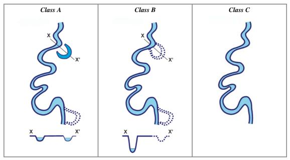
Figure 37 – Presence of typical fluvial forms in the alluvial plain. Class A: presence of natural fluvial forms (e.g. abandoned meander, oxbow lake). Class B: traces of fluvial forms, now disconnected by the channel due to incision, but with possible reactivation. Class C: complete absence of fluvial forms in the alluvial plain.
