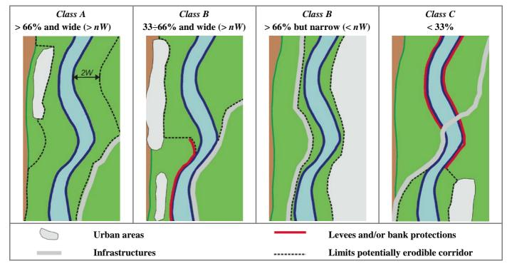
Figure 33 – Potentially erodible corridor. Class A: notwithstanding the constructed area and the road, a continuous and sufficiently wide erodible corridor exists. Class B: the erodible corridor is wide (mean width in the reach > nW) but with medium longitudinal continuity (33÷66%) (second figure from left), or it is continuous (> 66%) but not sufficiently wide (mean width < nW) (third figure from left). Class C: a potentially erodible corridor (of any width) exists only for < 33% of the reach.
