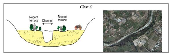
*Figure 29* – <u>CASE 5</u>: the channel is heavily incised (> 6 m) and narrowed, and the vegetation corridor has a medium width (F12 in  $Class\ B$ ). Field assessment enables verification that the vegetation in this case occupies portions of the 1954 channel disconnected by the present channel ("recent" terraces) ( $Class\ C$ ).
