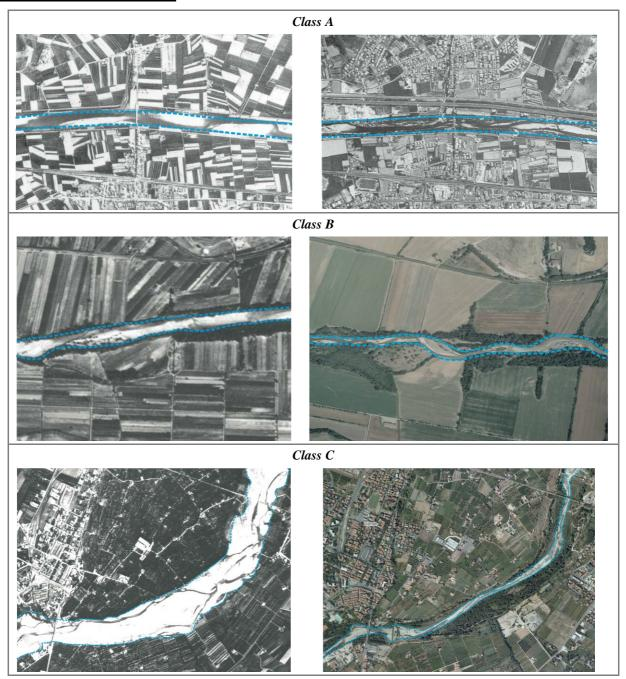
Figure 79 – Changes in channel width (on the left the aerial photo dated 1954, on the right the present situation). Class A: very limited channel narrowing (< 15%). Class B: channel narrowing from 15% to 35% of channel width in 1954. Class C: very intense channel narrowing (> 35%).
