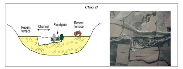
*Figure* 28 – <u>CASE 4</u>: the channel is incised and the vegetation corridor has a medium width (*F12* in *Class B*). Field assessment enables verification that most of the vegetations corridor corresponds to a modern floodplain formed after incision as consequence of lateral mobility (*Class B*).
