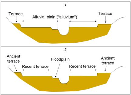
*Figure 22* – Distinction between alluvial plain and floodplain. (1) Terminology commonly used on geological maps; (2) terminology adopted here (the alluvial plain can include both floodplain and "recent" terraces, which are previous portions of a floodplain abandoned due to incision during the last 100÷150 years).
