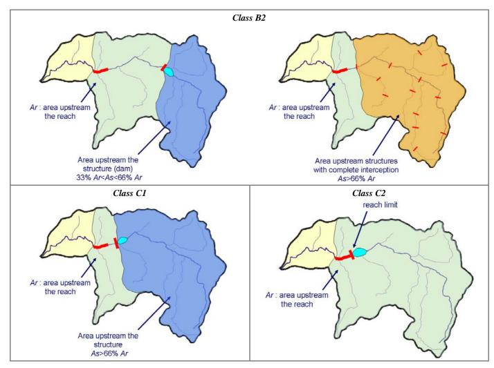
**Figure 57** (continued) – Upstream alteration of sediment discharges. Class B2: dam with a drainage area between 33% and 66% of the area upstream from the reach (left); the total area of portions of the watershed with check dams is > 66% of the area upstream from the reach (it applies in the case of reaches in hilly or lowland areas) (right). Class C1: dam with a drainage area > 66% of the area upstream from the reach (left). Class C2: dam at the upstream limit of the reach (right).
