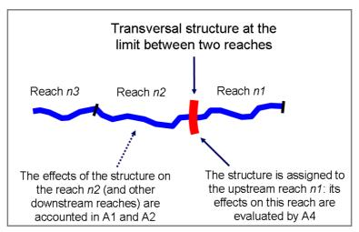
*Figure 51* – Rule of assignation of a transversal structure coinciding with the limit between two reaches and its effects on the alteration of sediment and water discharges.
