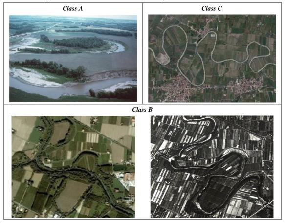
Figure 38 – Presence of typical fluvial forms in the alluvial plain. Class A: meandering river with a recent cut-off. Class C: meandering river with complete absence of forms in the plain. Class B: traces of abandoned meanders exits (photo on the left), disconnected from the channel because of bed incision. The observation of the aerial photos of the 1950's (photo on right) enables verification that these forms have been abandoned during the last decades.
