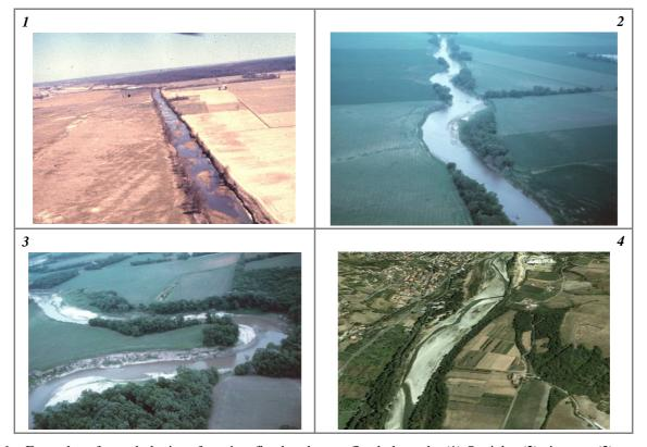
*Figure 6* – Examples of morphologies of semiconfined and unconfined channels. (1) Straight; (2) sinuous; (3) meandering; (4) sinuous with alternate bars.
