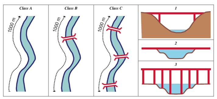
Figure 64 – Crossing structures. Class A: absence of structures. Class B: crossing structures in limited number ( $\leq 1$  every 1000 m). Class C: frequent crossing structures (>1 every 1000 m). On the right: interference of bridges with the fluvial corridor. (1) Bridge completely unrelated (viaduct crossing a valley at relevant height); (2) bridge with no piers but which may interfere with high discharges; (3) bridge very high but with piers interfering with fluvial dynamics processes.
