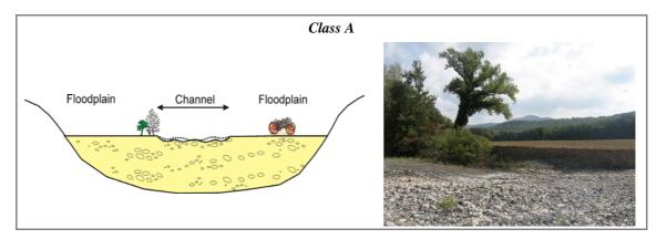
Figure 25 – CASE 1: the channel is not incised (V3 in  $Class\ A$ ), therefore the adjacent plain coincides with a modern floodplain ( $Class\ A$ ).
