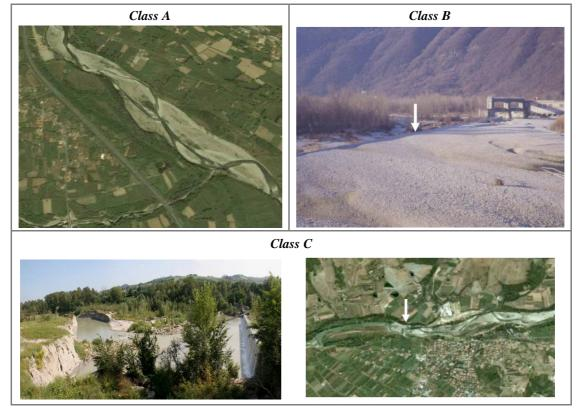
Figure 21 – Longitudinal continuity in sediment and wood flux. Class A: absence of discontinuities. Class B: filled check dam (arrow) altering the normal flux of sediment but without causing total interception and a discontinuity of forms (bars are equally existing either upstream and downstream). Class C: the presence of a weir or check dam with total sediment interception results in a significant alteration of the reach immediately downstream (the river flows from right to left).
