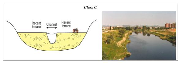
Figure 30 - CASE 6: the channel is heavily incised (> 6 m) and vegetation corridor that could be a post-incision floodplain is absent (F12 in Class C), therefore the reach is necessarily in Class C.
