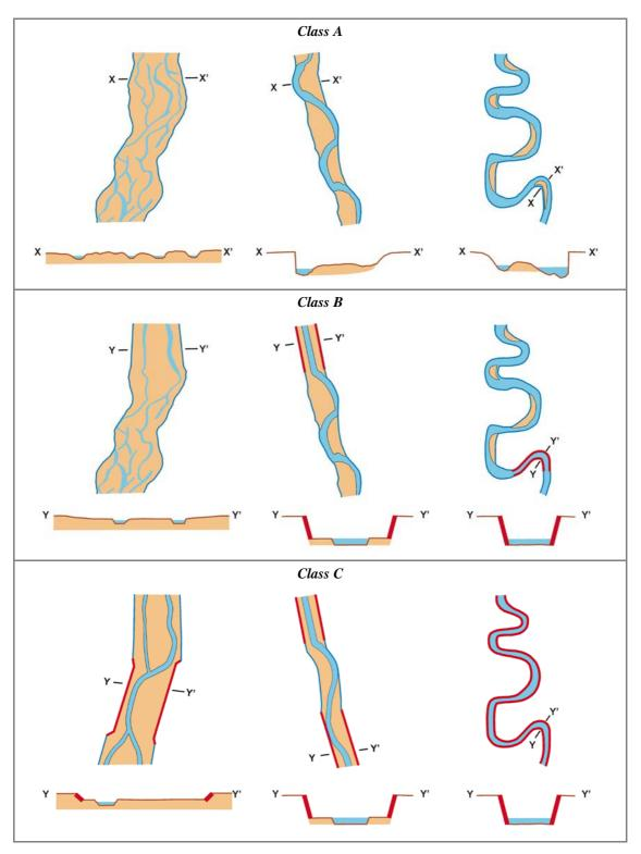
*Figure 41* – Variability of the cross-section in semi- and unconfined channels: examples for multi-thread, transitional, and single-thread channels. *Class A*: absence of alterations. *Class B*: alterations for a portion < 33% of the reach length. *Class C*: alterations for a portion > 33% of the reach length.
