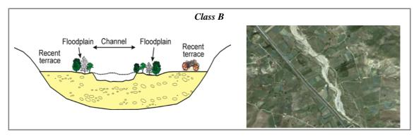
Figure  $26 - \underline{\text{CASE } 2}$ : the channel is slightly incised and narrowed compared to 1954. Vegetation in the fluvial corridor is quite wide (F12 in Class B) and mostly coincides with the channel of 1954. The field assessment enables verification that the vegetation corridor coincides with the modern floodplain, resulting therefore in Class B.
