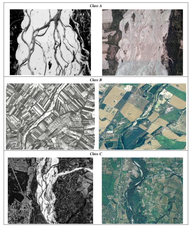
*Figure* 78 – Changes in channel pattern (on the left the aerial photo dated 1954, on the right the present situation). *Class A*: the channel maintains a prevailing braided pattern, although channel narrowing occurred. *Class B*: change from wandering to sinuous. *Class C*: change from braided to sinuous.
