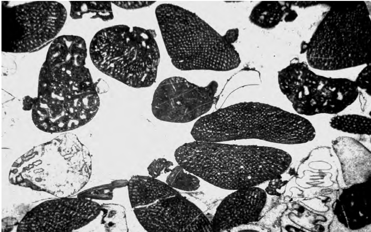
Fig. 1 – Rudstone con Orbitolina ( Mesorbitolina ) texana , Coscinophragma cribrosum , Nerineidae e resti di Scleractinia . x 20 – Rudstone with Orbitolina ( Mesorbitolina ) texana , Coscinophragma cribrosum , Nerineidae and Scleractinia remains. x 20
