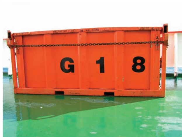
Figure 3. A SANAP container on the main forward deck of the S.A. Agulhas, showing two fork-lift slots in its base that are accessible to mice. Photo: John Cooper
