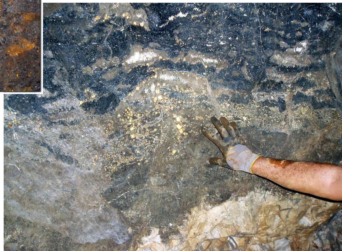
Fig. 11 - Pyrite, chalcopyrite and pyrrhotite ore in hedenbergite-ilvaite skarn; Temperino mine.
