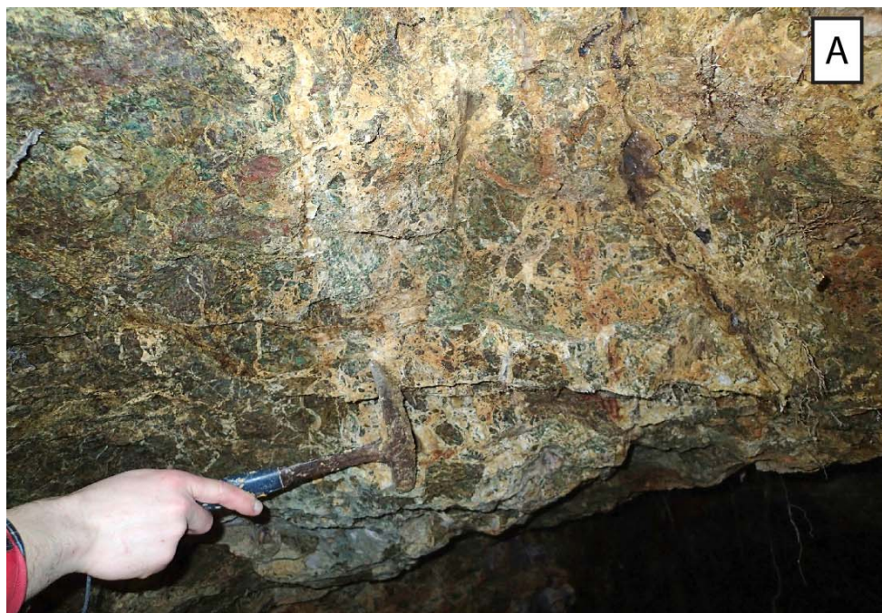
Fig. 62 – (A) On the left an example of brecciated and carbonated serpentinite, infilled by dolomite veins; (B) On the right, brecciated magnesite vein, partially cemented by dolomite and silica.
