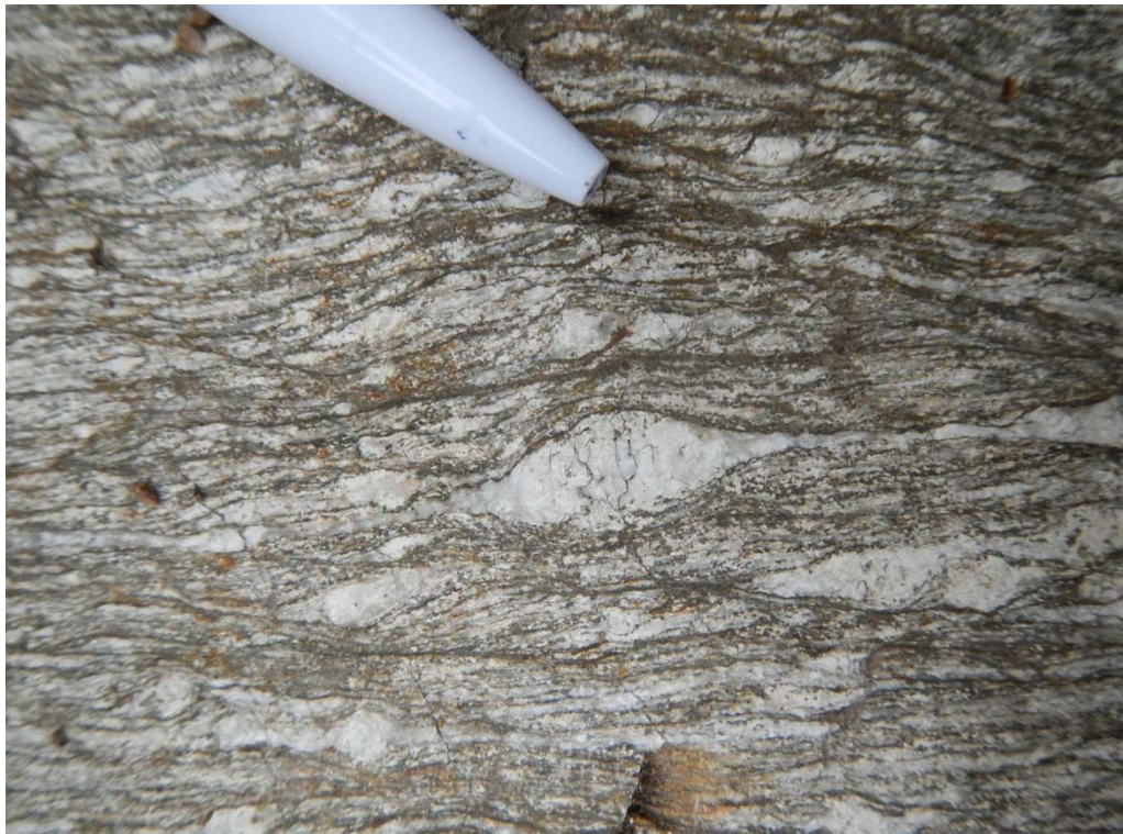
Fig. 1.28 - C-S fabric and sigma-type porphyroclast showing a top-to-the NW sense of shear in the augen gneiss.
