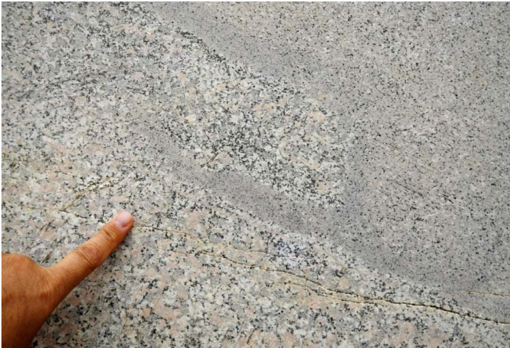
Fig. 4.6 - Detail of the magmatic contact between a coarse-grained granodiorite (bottom) and a fine-grained granite (top) shown in the quarry cut of Fig. 4.5. of the Arzachena pluton.
