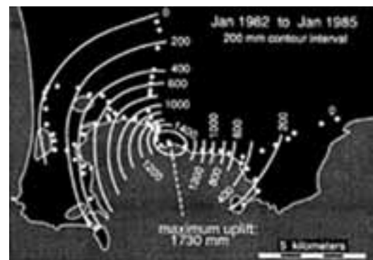
Figure 11 - Results of levelling surveys conducted between January 1982 and January 1985. The isolines of ground deformation are in mm (Dvorak and Mastrolorenzo, 1991).
