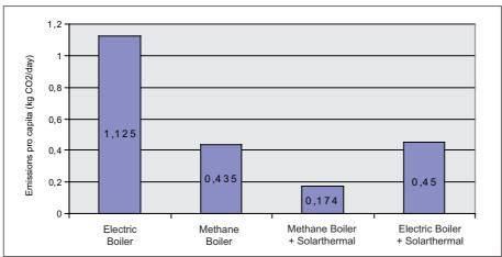
Figure 2. Assesment of  ${\rm CO_2}$  emissions generated by different systems (ISES)
