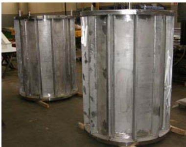
Fig.2. Two shielded containers for activated MTR terminals.
