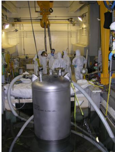
Fig.3. Sludge collection vessel.
