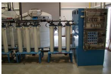
Fig. 4. Electro coagulation cells.
